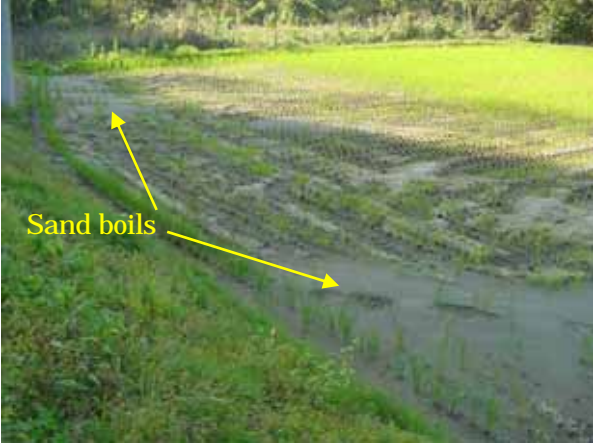
Scattered sand boils were seen in farm lands at several locations of the investigated area.
