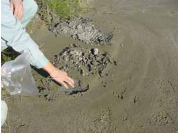
Scattered sand boils were seen in farm lands at several locations of the investigated area.
