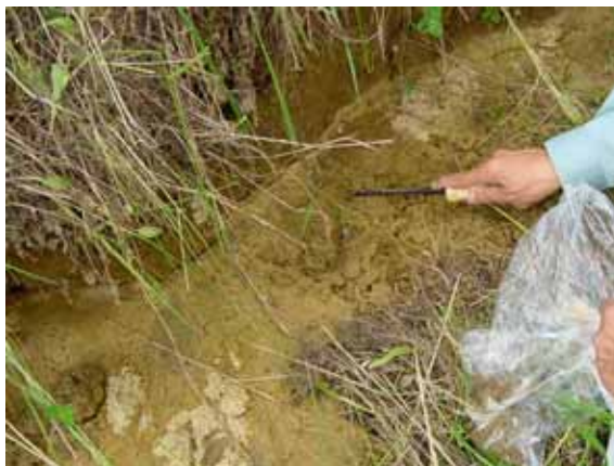
Onbetsu: The fill soils are sandy soils; liquefaction of the relatively loose fills is considered to be the cause of the observed damage as above; (B-1)
