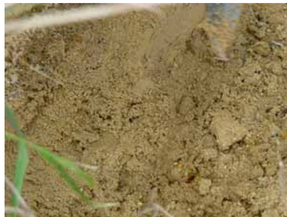
Onbetsu: The fill soils are sandy soils; liquefaction of the relatively loose fills is considered to be the cause of the observed damage as above; (B-1)
