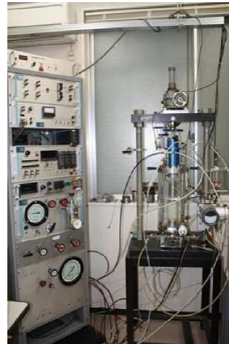
Triaxial Compression Test on Unsaturated soil
