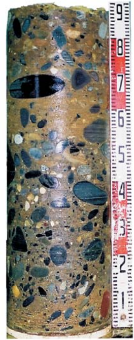
SAMPLED BY GP-R (300mm dia.) GRAVELS AND FINES
