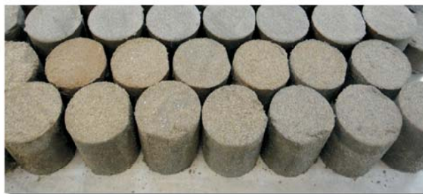
Photo 2 : Self-standing sand samples after extrusion from the sample tubes. They are sampled by GP-S.
