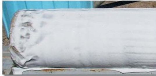
Photo 1 : GP Sample which is covered with polymer gel.
