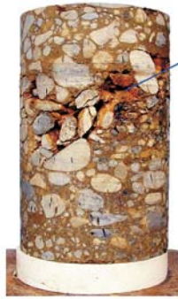
SAMPLED BY GP-D (200mm dia.) GRAVELS WITH SAND
