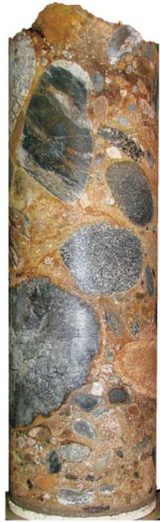
SAMPLED BY GP-R (300mm dia.) VERY HARD GRAVELS WITH LOOSE SANDS
