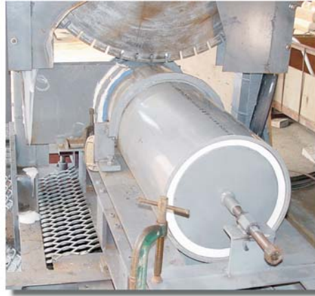
A sample case for cutting & large cutter with polymer solution.
