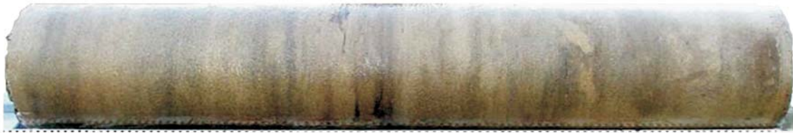
SAMPLED BY GP-D (200mm dia.) GL-16.10 - 17.15m SANDY MATERIAL LAYER
