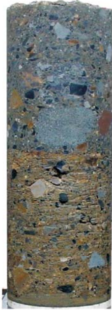
SAMPLED BY GP-R (300mm dia.) FILL MATERIAL FOR A ROAD
