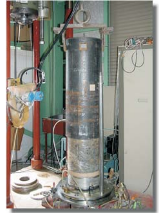
A carrying case & a triaxial test apparatus for 300mm dia. specimen.
