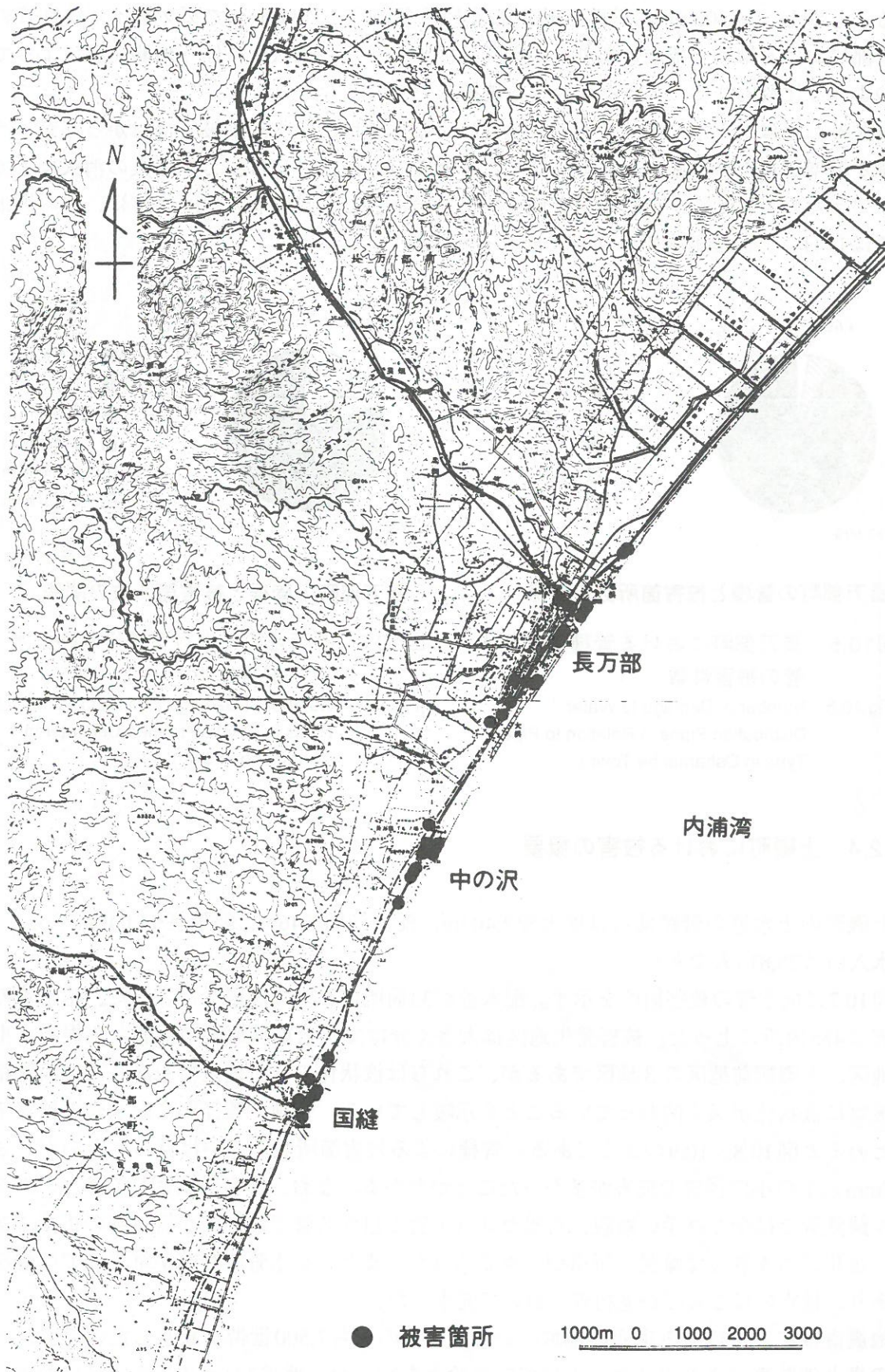
図10.4 長万部町の配水管の被害分布 (Fig.10.4 Distribution of Damage to Water Distribution Pipes in Oshamanbe Town)
