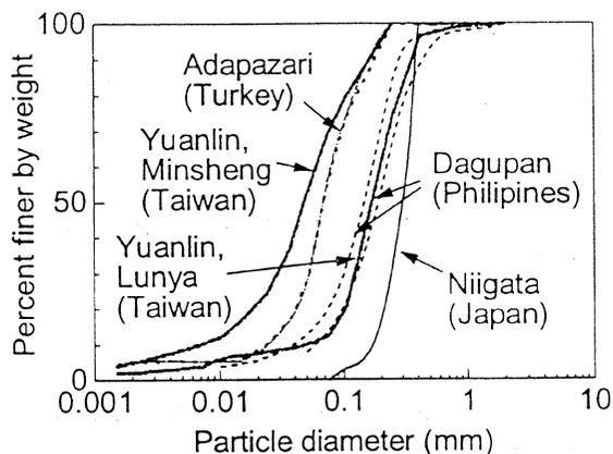
Fig.7 Grain size distribution curves of liquefied soils in four cities
