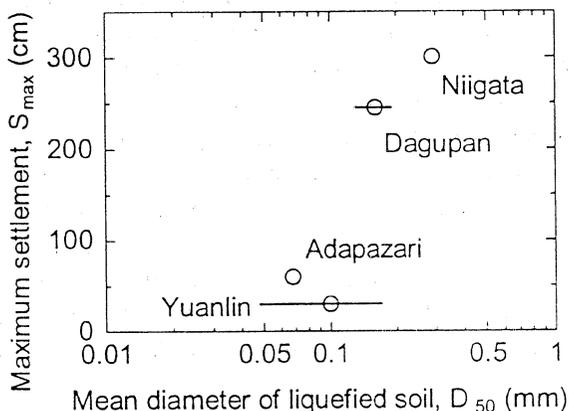
Fig.8 Relationship between mean diameter of liquefied soil and maximum settlement of buildings
