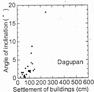
Fig.5 Relationship between angle of inclination and settlement of the selected buildings with spread foundations in Dagupan City (Yasuda, 2000)
