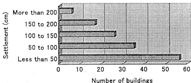
Fig.1 Frequency distribution of the settlement of damaged buildings in Niigata City (Building Research Institute, 1965)
