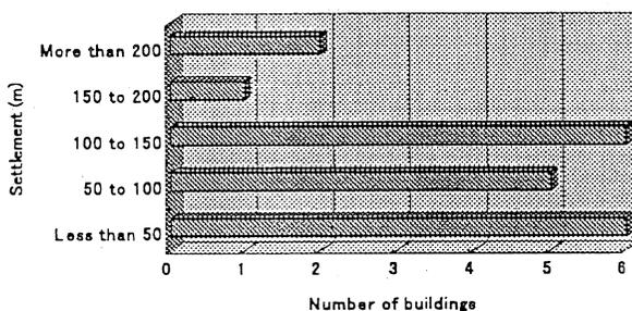
Fig.2 Frequency distribution of the settlement of selected buildings with spread foundations in Niigata City (Yasuda, 2000)
