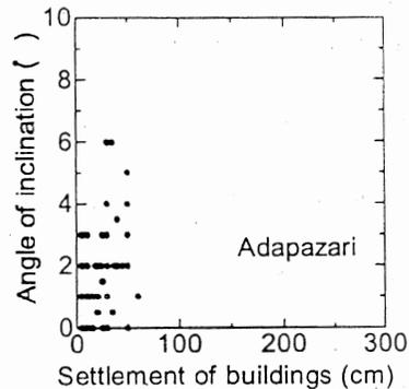
Fig.6 Relationship between angle of inclination and settlement of the investigated buildings in Adapazari (Yasuda, 2000)
