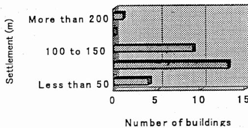
Fig.4 Frequency distribution of the settlement of selected buildings with spread foundations in Dagupan City (Yasuda, 2000)
