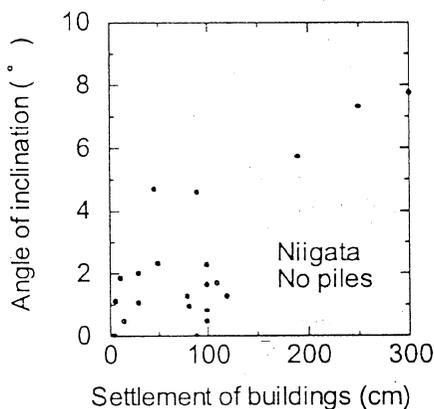
Fig.3 Relationship between angle of inclination and settlement of the selected buildings with spread foundations in Niigata City (Yasuda, 2000)
