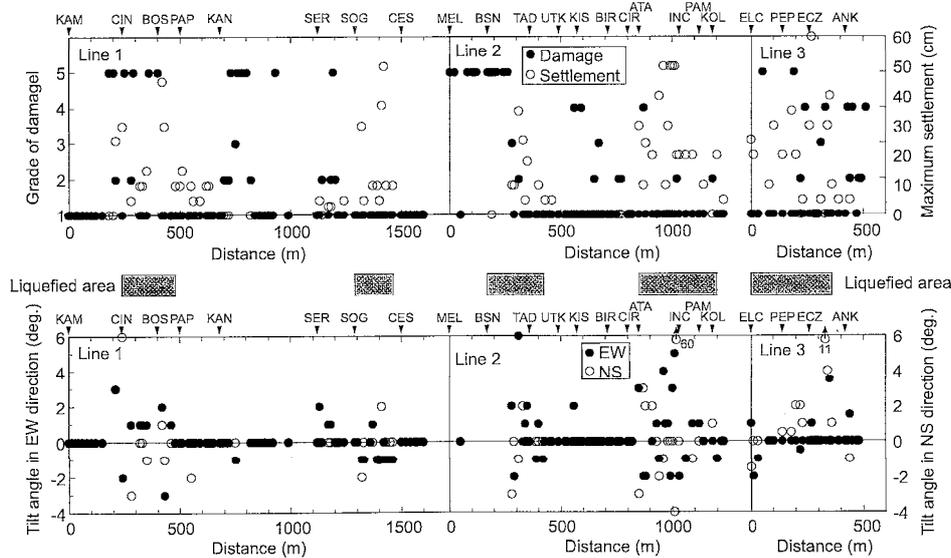
Fig. 9. Results of detailed damage investigation
