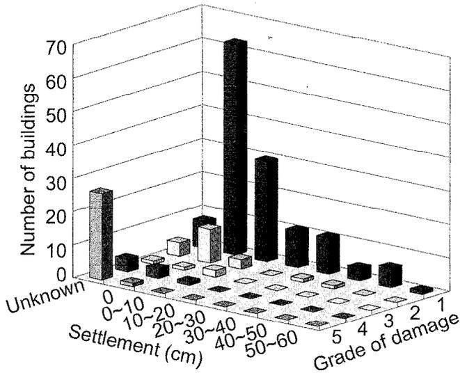
Fig. 11. Relationship between settlement and grade of damage
