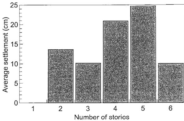
Fig. 12. Effects of number of stories on settlement of buildings in liquefied area
