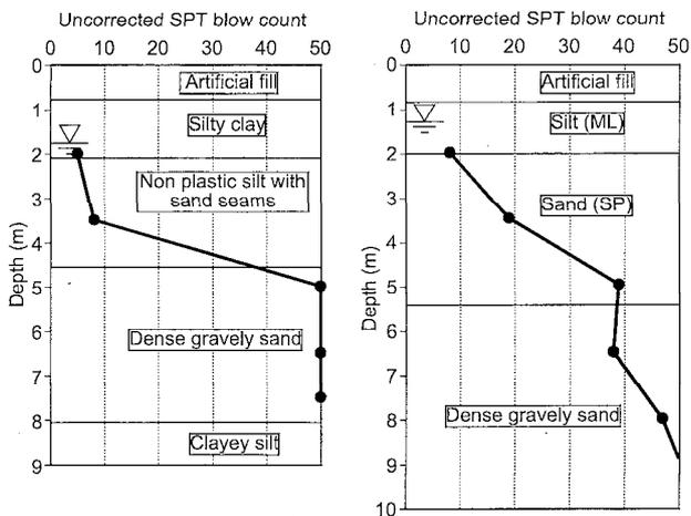
Fig. 4. Drilling log along the Cark Cadesi (Modified from Erken, 1999)
