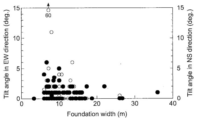
Fig. 14. Relation between angle of tilt and foundation width of buildings in liquefied area
