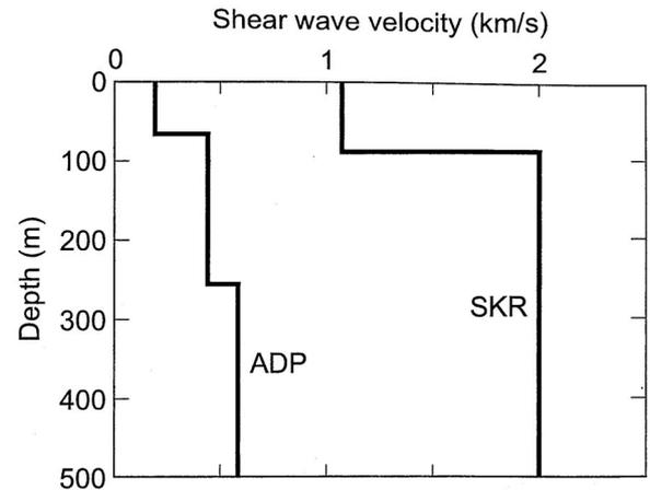
Fig. 2. Shear wave velocity identified from microtremor measurement
