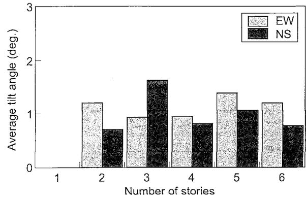
Fig. 13. Effects of number of stories on tilt of buildings in liquefied area
