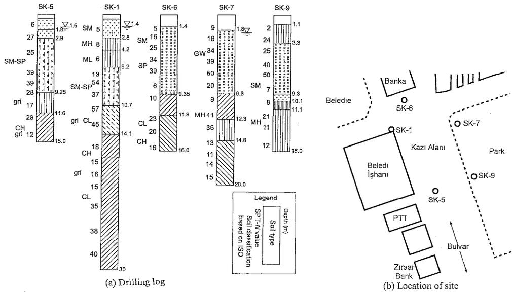
Fig. 5. Drilling log north from station (Modified from Onalp, 1999)
