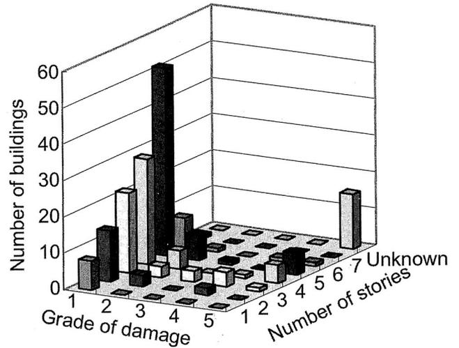
Fig. 10. Relationship between grade of damage and number of stories
