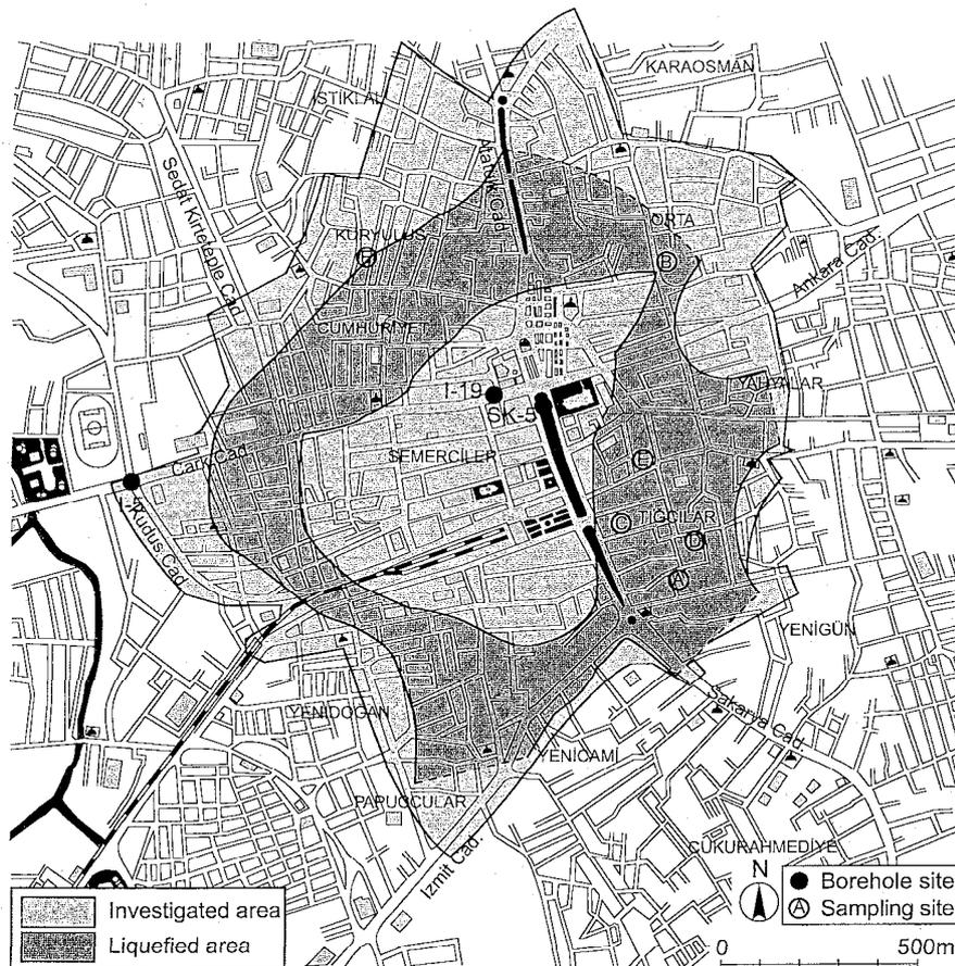
Fig. 3. Map of downtown Adapazari: Investigated area, site of borehole investigation, sand sampling, and liquefied area
