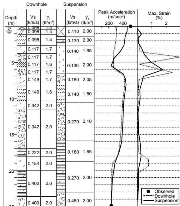
Figure 7. Peak acceleration and maximum strain distribution
