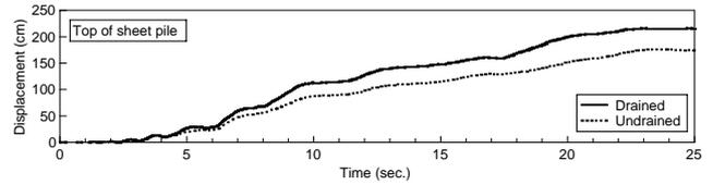
Figure 3 Horizontal displacement at the backfill of the ground under drained and undrained conditions. (modified from ref. 6)
