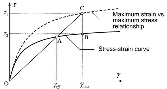
Figure 13 Schematic figure showing the mechanism of the overestimation of the shear stress by the equivalent linear method.
