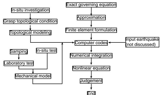
Figure 1 Flow of the dynamic response analysis to obtain final result
