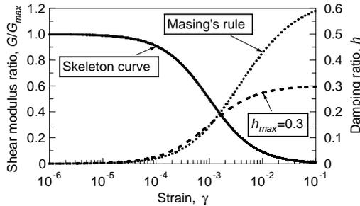
Figure 11 Error of damping ratio by Masing's rule
