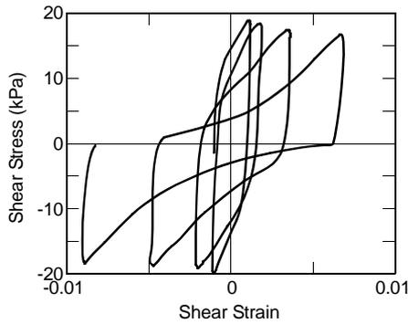
Figure 10 Stress-strain curves at large strains. Hysteresis curves does not become stable at large strains.
