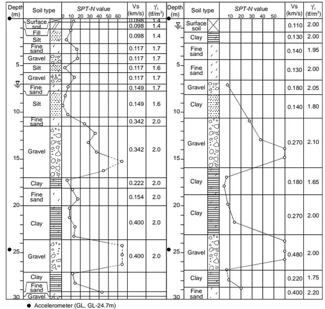
(a) Before earthquake (downhole) (b) After earthquake (suspension)
