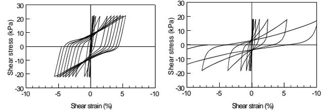
(b) Example of stress-strain curve
