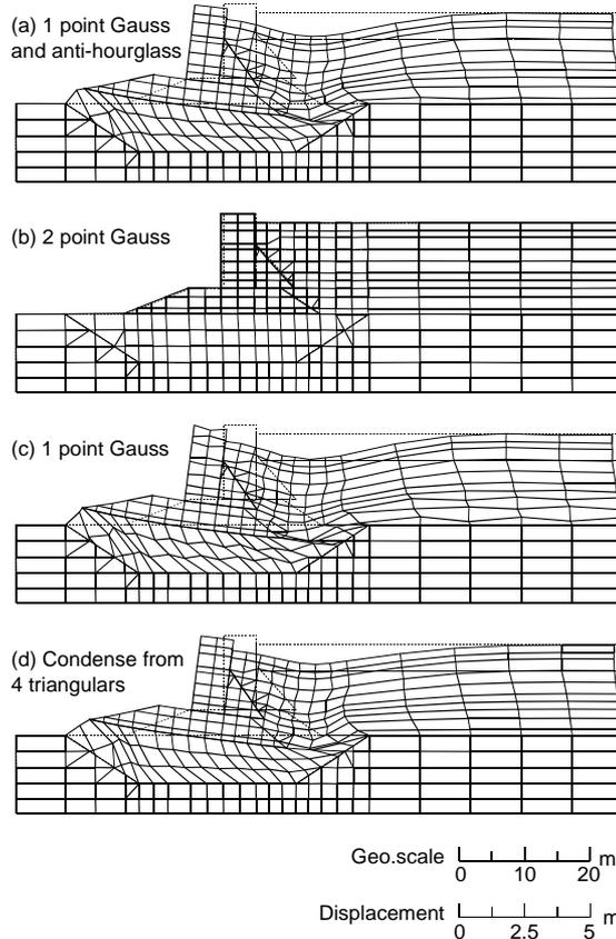
Figure 4 Shear locking, hourglass instability and its solution
