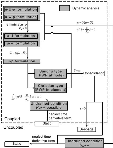
Figure 2 Biot's equation: accurate and approximate formulation including consolidation and static formulations.
