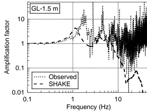
Figure 14 Underestimation of amplification factor by SHAKE
