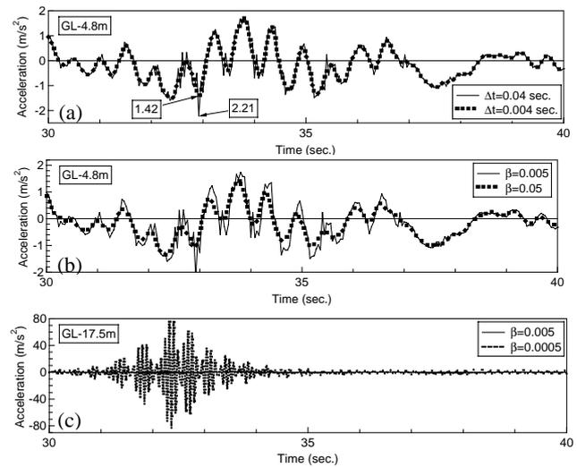
Figure 5 Example of pulse response. (a) Pulse wave at about 33 seconds (b) Elimination of pulse by larger damping (c) Many pulse waves by smaller damping
