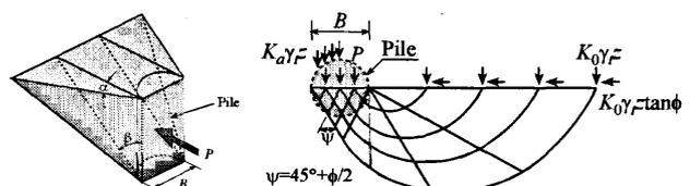
Figure 6 Mechanisms at ultimate state
