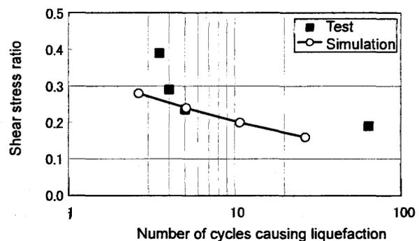
Figure 9: Simulation of liquefaction strength
