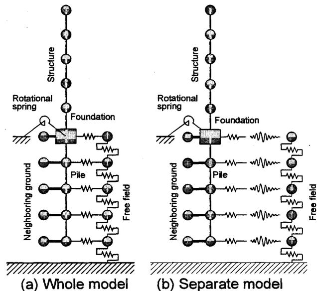
Figure 1 Soil-pile-structure model
