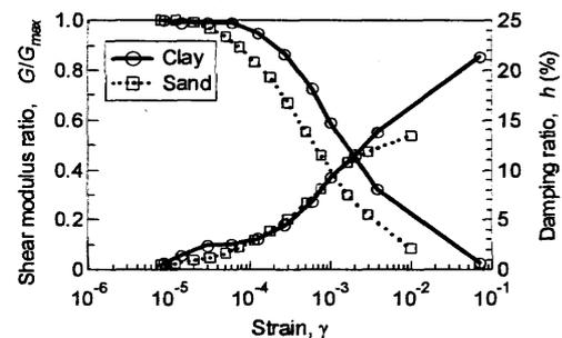
Figure 5: Dynamic deformation characteristics
