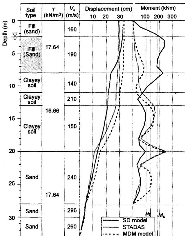
Figure 17: Ground displacement and bending moment of pile
