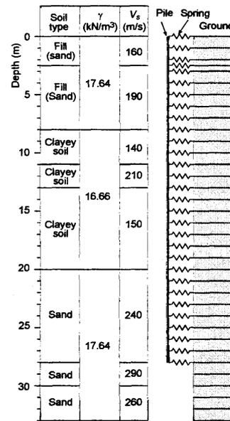
Figure 4: Structural model and soil parameter
