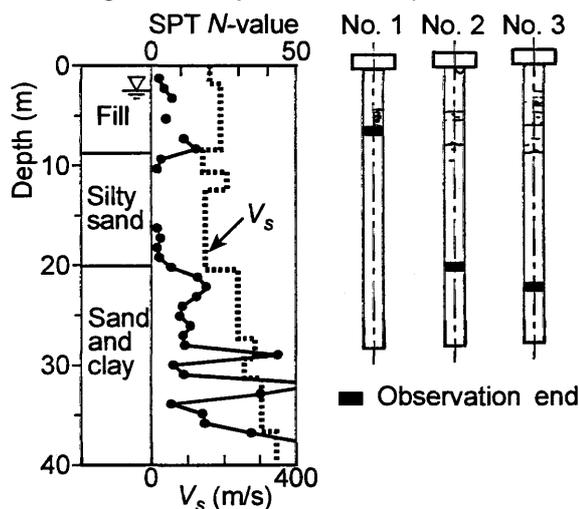
Figure 2: Soil profiles and damage to piles
