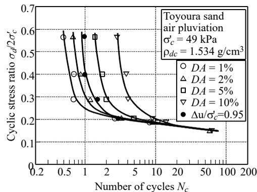
Fig. 2 Example of liquefaction strength test (JGS, 2020).
