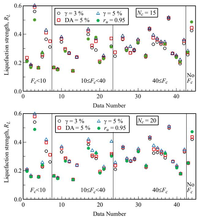
Fig. 4 Liquefaction strengths for  $N_c = 15$  and  $20$ .
