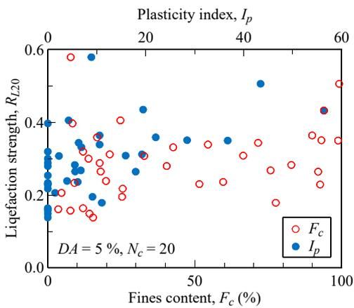
Fig. 7 Liquefaction strength depending on  $F_c$  and  $I_p$
