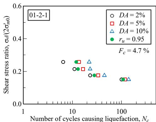
Fig. 9 Liquefaction strength of test 01-2-1 ( $F_c = 4.7\%$ )
