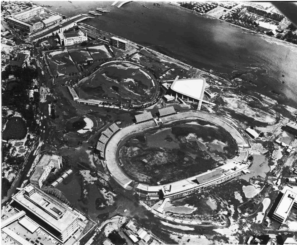
Fig. 33. Liquefaction around the sports complex near the Showa Bridge (still photo taken by Mr. Yuminamochi) 競技場地区
