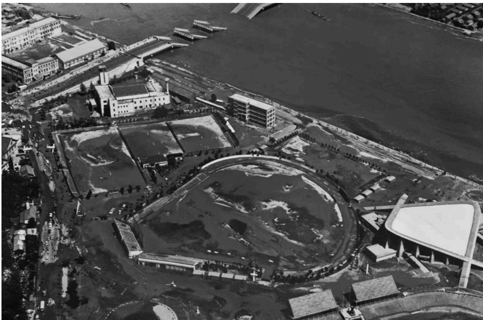
Fig. 34. Liquefaction in and around the baseball stadium (still photo taken by Mr. Yuminamochi) 野球場周辺の被害状況
