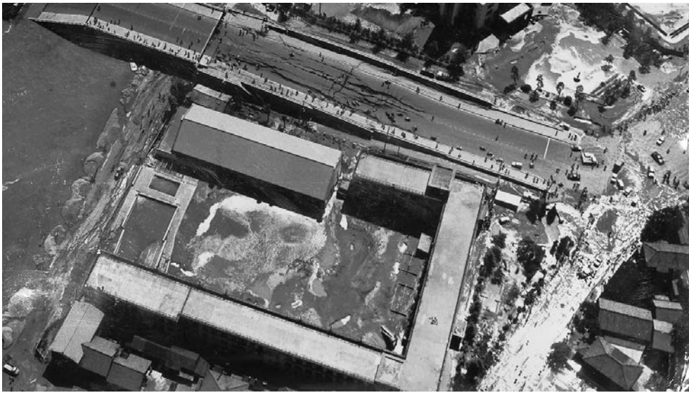
(b) Details of liquefaction damage in the Hakusan Elementary School 白山小学校被災の詳細
