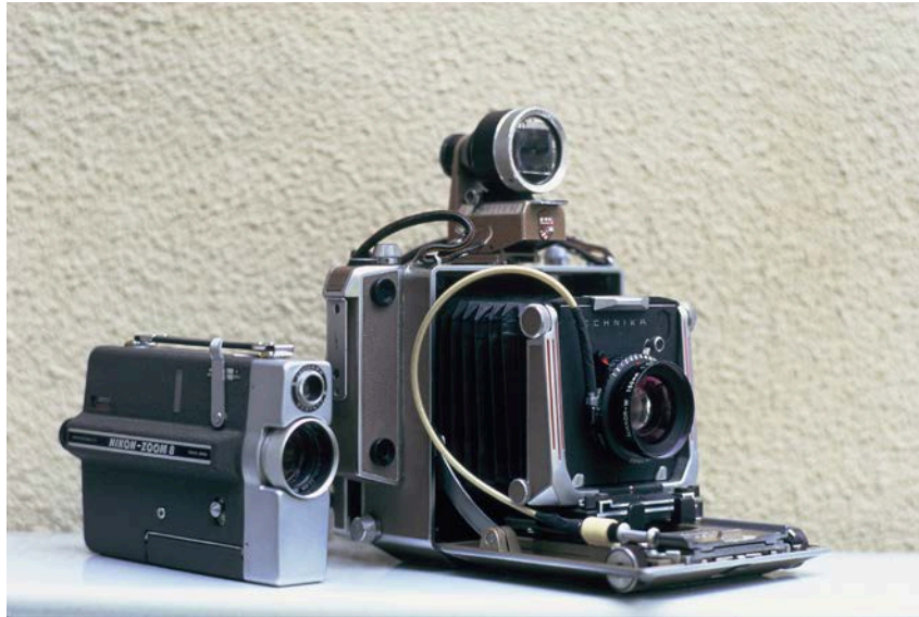
Fig. 4. Mr. Yuminamochi's Nikon 8-mm movie camera (left) and Linhof Technika still large-format camera (right) for color photographs with 4' × 5' film with 150-mm lens (he had two more cameras that were Speed Graphic for black-and-white 4' × 5' photographs with 127-mm lens and Asahi Pentax with 35-mm and 135-mm telescope lenses) (photograph provided by Mr. Yuminamochi) 弓納持氏の使用したニコン8ミリ撮影機とリーnhof・テクニカカメラ (弓納持氏提供の写真)
