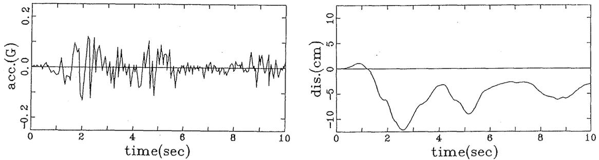
Fig. 3 Acceleration and Displacement Time Histories of Incident Wave
