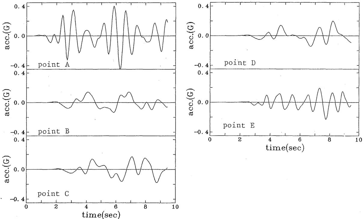
Fig. 4 Acceleration Response at the Surface
