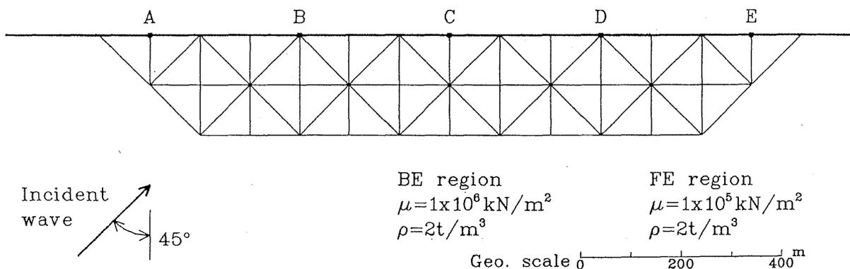
Fig. 2 Alluvial Valley Model, Finite Element Mesh and Material Properties
